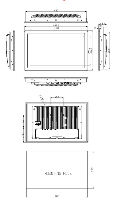
**Note:** Dimensions are in mm (Tolerance ±0.5 mm).
